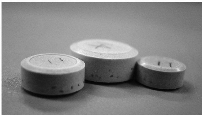
Fig. 5. Sample tablets with pellets exuding from the side. The white on the side of the tablet is diluent, while the colored particles dotted on the lower surface are pellets.
